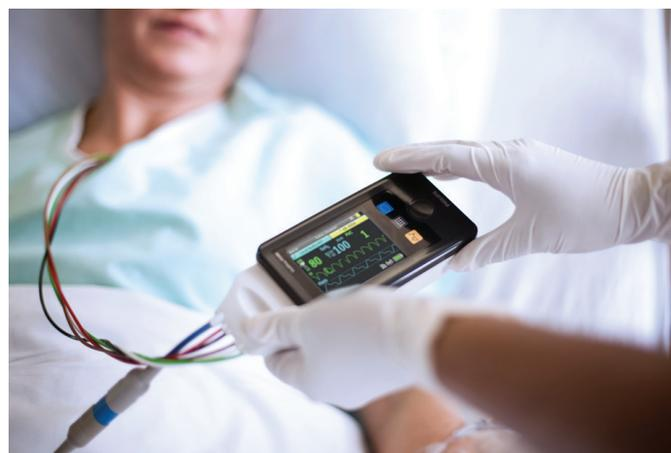
**Figure 1.** The Philips IntelliVue MX40 wearable patient monitor.
